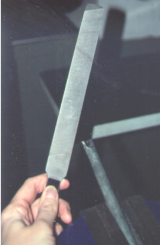
Figure 27: Filing of knife-edge
