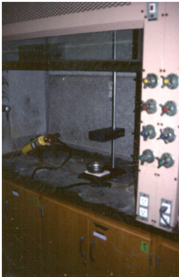
Figure 33: Torching setup inside fumehood
