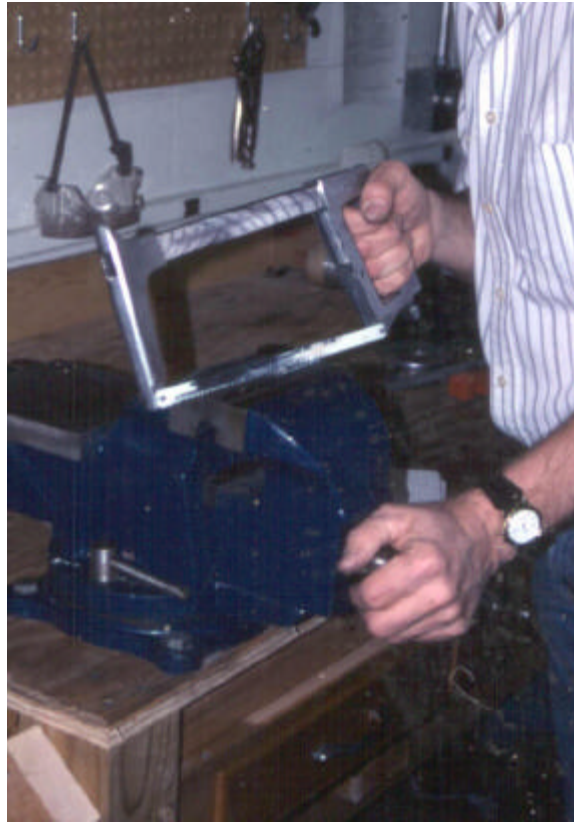
Figure 30: Sawing of bolt for upper crosspiece
