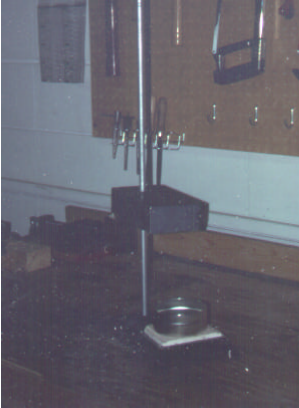
Figure 31: Setup for melting of lead brick
